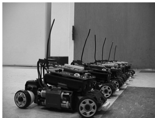
Figure 1. A line of CotsBots. Over 80 robots have been built to date.
